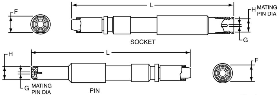
NOTE: All contacts of the same size and the same inner and outer contact diameters (G & H) will mate with each other.
