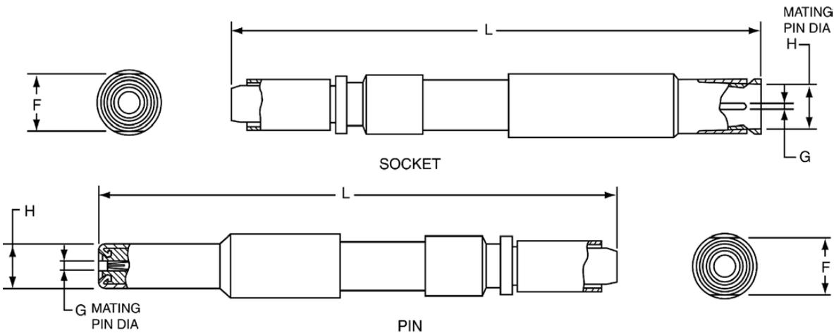
NOTE: All contacts of the same size and the same inner and outer contact diameters (G & H) will mate with each other.
