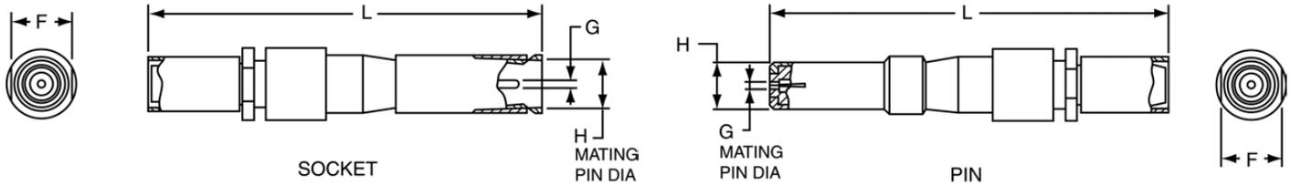
NOTE: All contacts of the same size and the same inner and outer contact diameters (G & H) will mate with each other.
