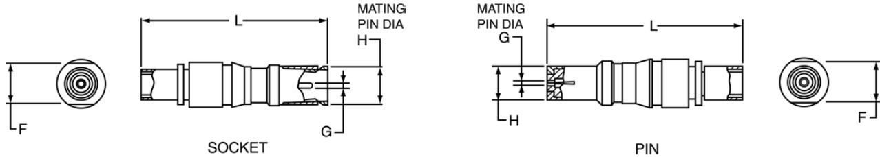
NOTE: All contacts of the same size and the same inner and outer contact diameters (G & H) will mate with each other.
