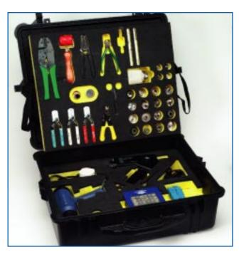
The Amphenol Fibre Optic Termination Kit is specified as a generic termination system which includes all the necessary basic tooling equipment.
