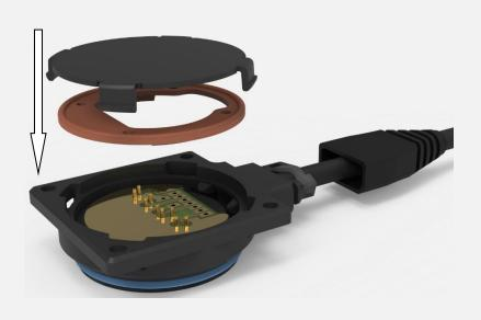
PLACE THE SEAL ONTO THE REAR PLATE AND CLIP REAR PLATE INTO THE RECEPTACLE, SLIDE OVER BOOT UNTIL SECURED
